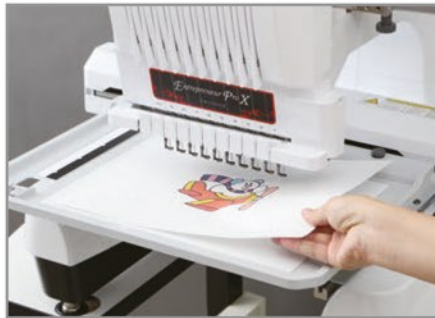
Set printed image on the frame
