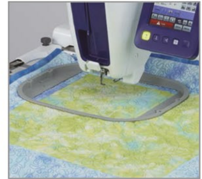
The PRS100/VR offers a 200 mm × 200 mm sewing range
